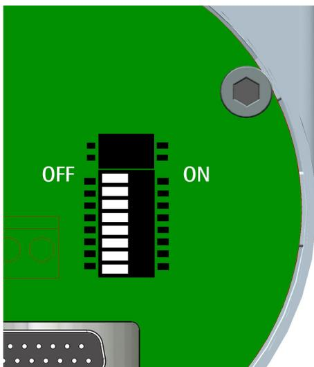
The node address must be set via hardware using the DIP A dip-switches located inside the connection cap.
