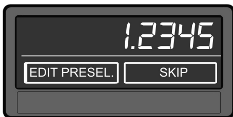
Display for quick start of the preselection values setting process (see the "6.10 Preselection values menu" section on page 63)
