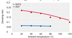
\*Although the damping ratio and dynamic rigidity decrease as the temperature rises, **XGT2** exceeds the damping ratio and dynamic rigidity of **XGT** across the entire temperature range.
