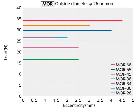
These are initial slippage load values of hubs and a spacer.
