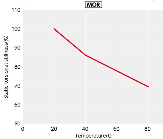
This is a value under the condition where the static torsional stiffness at 20°C is 100%.
