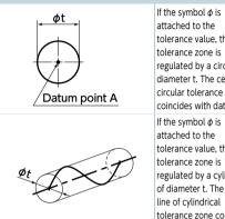
tolerance zone is regulated by a circle of diameter t. The center of circular tolerance zone coincides with datum A If the symbol  $\phi$  is attached to the tolerance value, the tolerance zone is regulated by a cylinder of diameter t. The axis line of cylindrical tolerance zone coincides with datum A.
