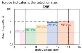
• Selection example In case of selected parameters of shaft diameter of  $\phi$ 14 and load torgue of 9 N·m, the selected size is
