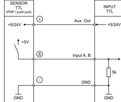
Unconnected PNP inputs are always "LOW" and unconnected NPN inputs are always "HIGH".
