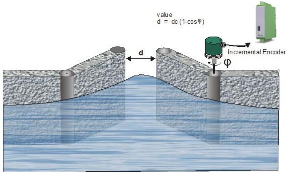
In this case we need to convert a non-linear input signal (incremental encoder signals  $\varphi$ ) into a linear representation (opening of the gate "d"). In the x-axis we must set the actual values detected by the encoder while in the y-axis we will set the opening values of the gate.
