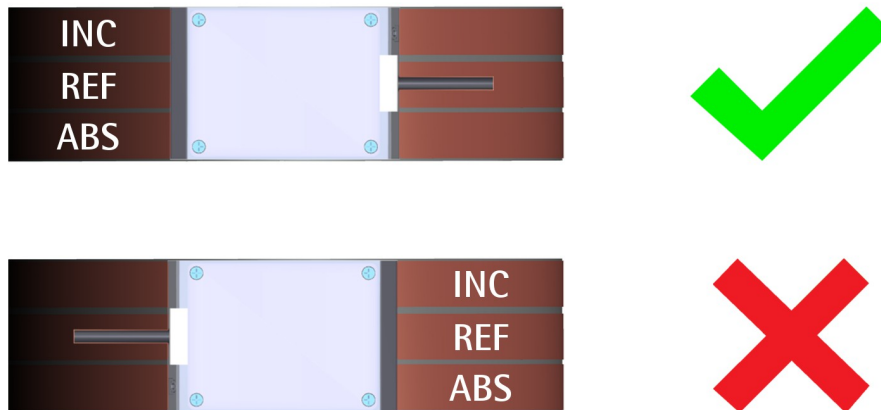
Figure 5 - Mounting direction of the sensor
