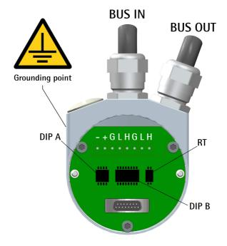
The connection cap of PG versions (CC-CB connection cap) is fitted with two PG9 cable glands for BUS IN, BUS OUT, and power supply connections. The bus cables can be connected directly to the terminal connectors located in front of each cable gland. We recommend CANbus certified cables to be used. Core diameter should not exceed Ø 1.5 mm (0.06 inches).
