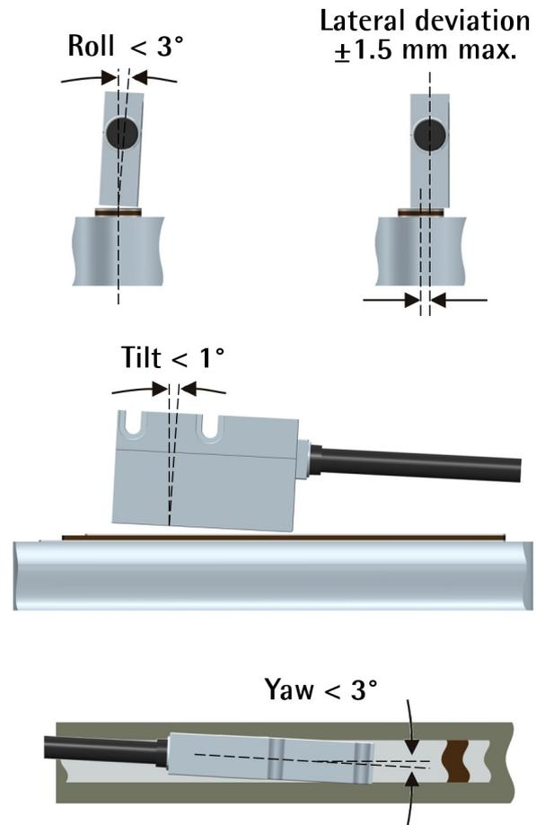
Figure 2 - Sensor / scale mounting tolerances
