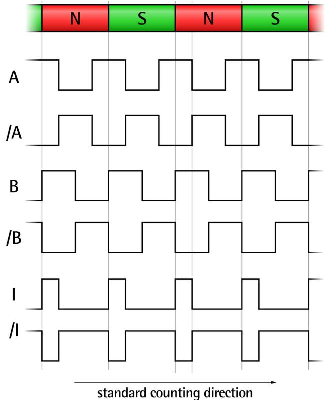
Figure 5 - Example with interpolation factor 4x
