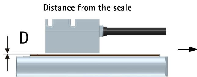
Figure 1 - Sensor / scale mounting gap
