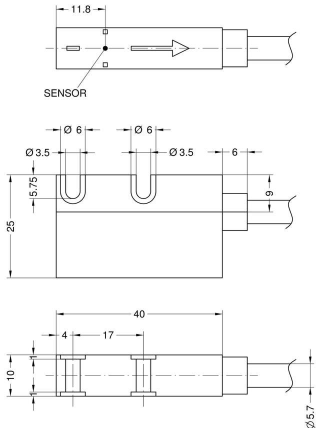
**3.2 Mounting the sensor with magnetic scale**
