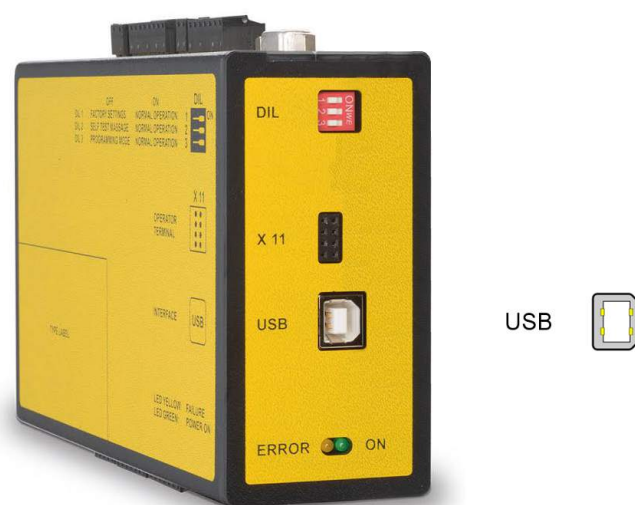
Figure 30 - [USB] type B USB port
