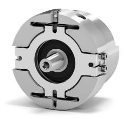
ASB62 is the absolute rotary encoder for position and speed feedback on gearless and servo motors. Tapered solid shaft and expansion flange provide easy and secure installation and eliminate shaft slippage.
